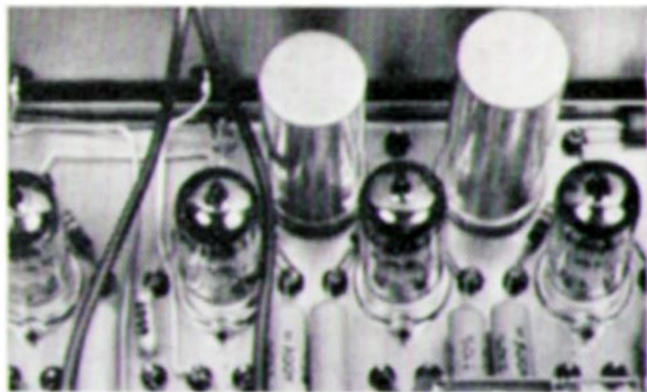
Four special low-noise ECC807 twin-triodes employed in input and tone compensation stages.
