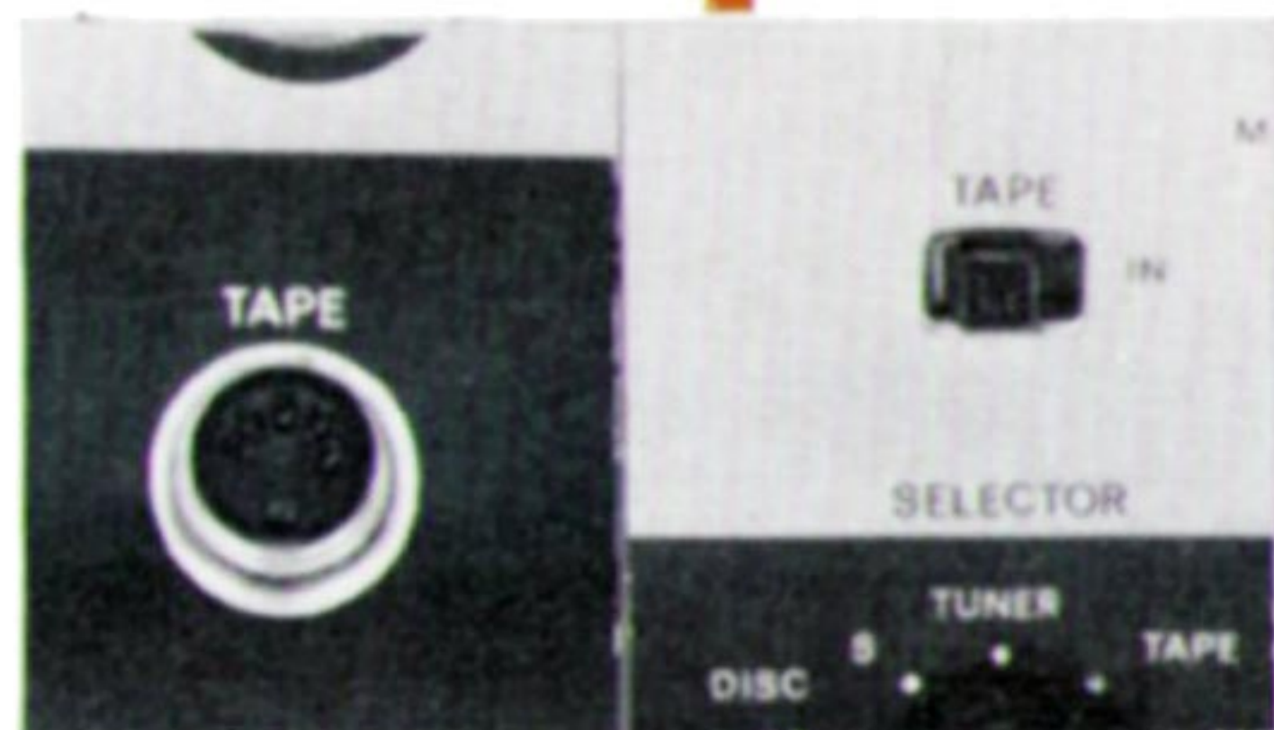
5-pin DIN Panel Socket for complete Tape Recorders. Tape slide-switch provides monitoring and speaker muting facility.
