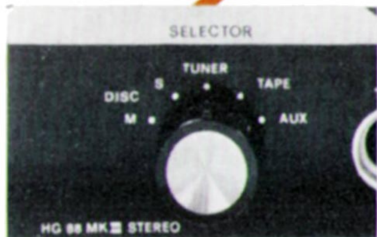
5-position Input Selector provides Disc, Tuner, Tape and Aux settings. Mono Disc setting for compatible stereo cartridges.
