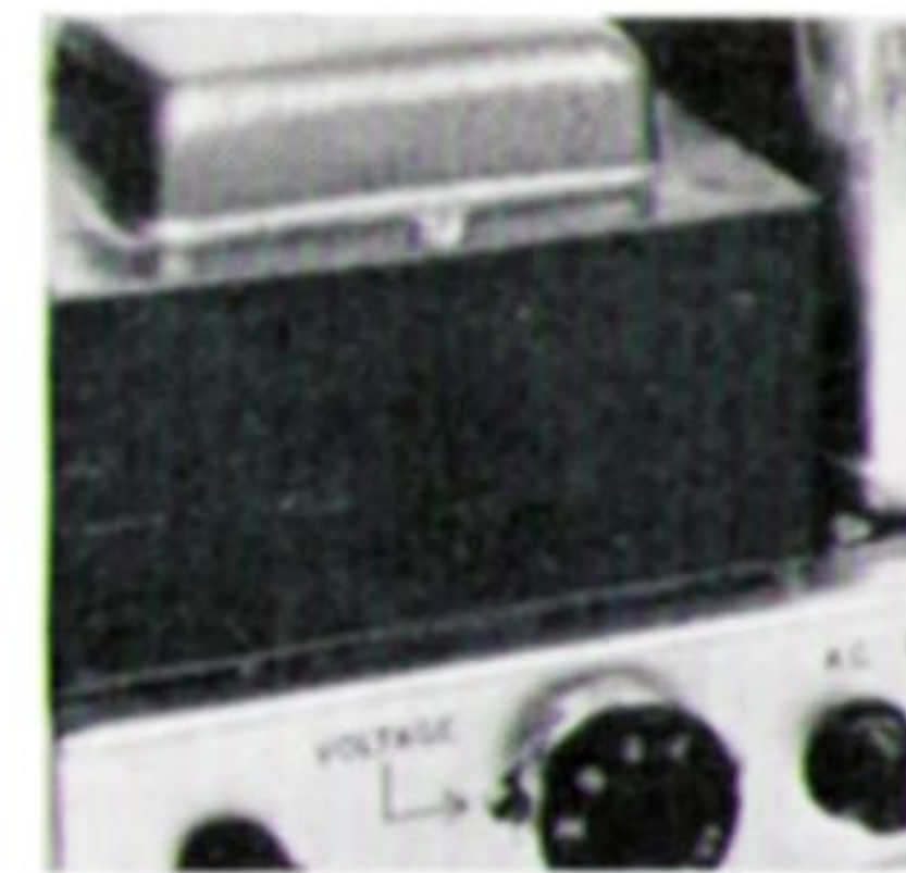
Dual voltage double-wound mains transformer.
